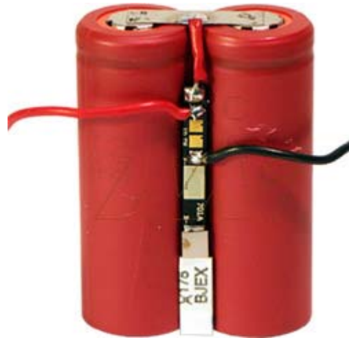
Sanyo 2/UR18650F in parallel fitted with PCM and SRP175 polyswitch
