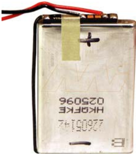
Sanyo UF553450F cell fitted with PCM
