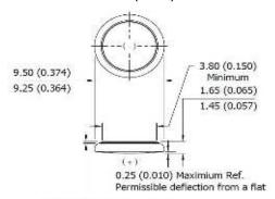
0.02 (0.001) Minimum Ref. (applies to top edge of gasket or edge of crimp, whichever is higher)
